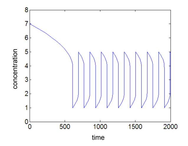
From different initial conditions, the system reaches the limit cycle and oscillates with the same frequency and amplitude.
