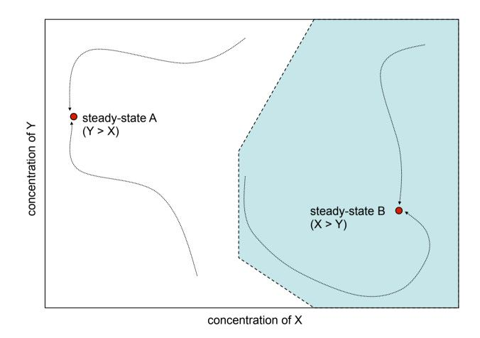
The system tends to either steady-state A or steady-state B depending on the initial conditions.
