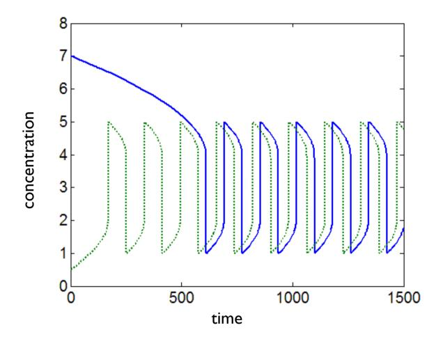
The time taken to reach the limit cycle is different for different initial conditions.
