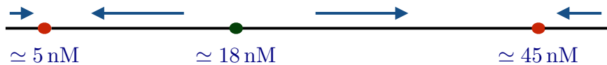
Figure 5: The phase portrait when [p] = 20 \text{ nM} (see Fig. 6). If the initial [\text{Mos}] is above the value at the unstable steady state, then [\text{Mos}] tends to the upper stable steady state. If the initial [\text{Mos}] is below the value at the unstable steady state, then [\text{Mos}] tends to the lower stable steady state.
